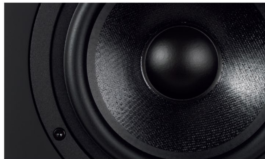
The cone membrane of the Type 07’s sub/midwoofer is made of an Ultra Honeycomb Composite, an ultra-light but rigid sandwich membrane composed of a Kevlar texture (outside) and a Kapton honeycomb structure (inside).
